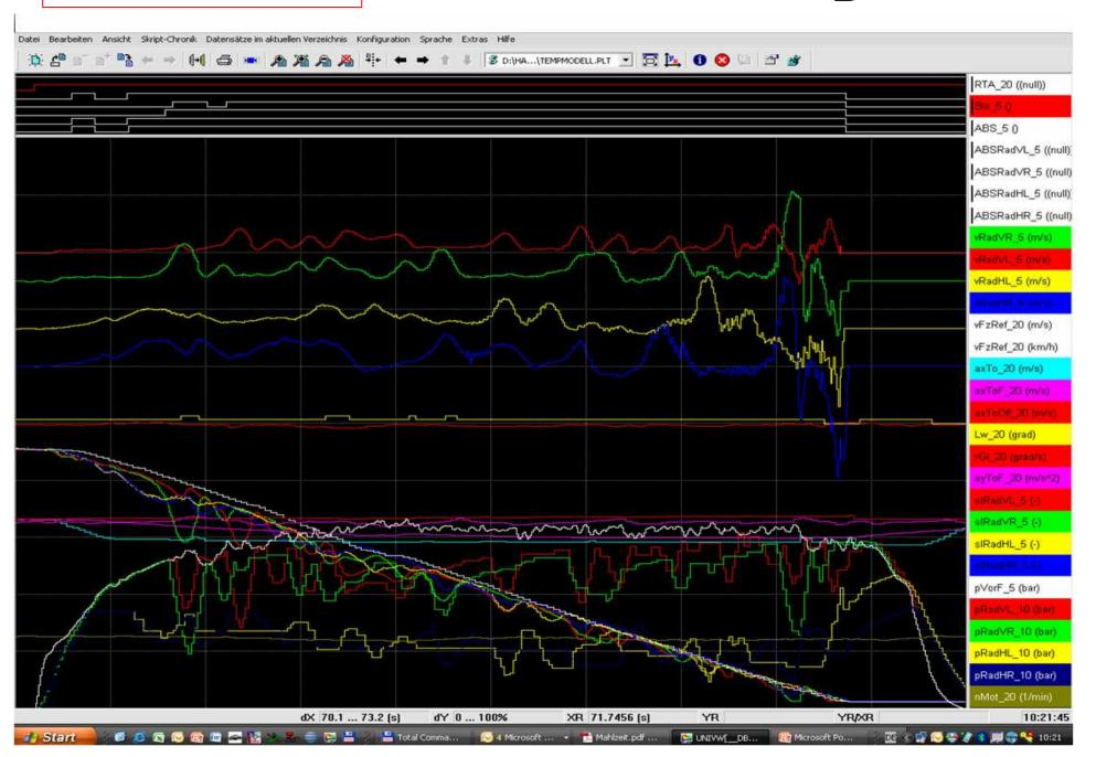
Comparison of  $\mu$ -slip characteristics on drum (d=2,547m)
