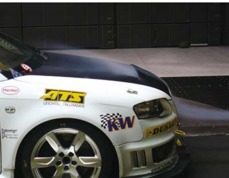
Design of the CFRP hood with integrated air outlet including aerodynamic optimization in SC/Tetra (above, right) and wind tunnel testing the aero settings for 2010 at FKFS in Stuttgart (left)
