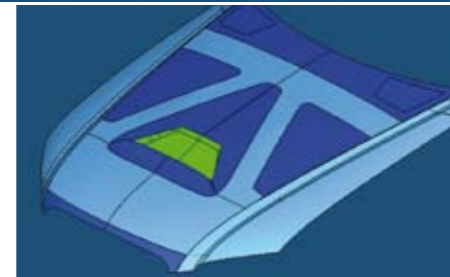
Design of the CFRP hood with integrated air outlet including aerodynamic optimization in SC/Tetra (above, right) and wind tunnel testing the aero settings for 2010 at FKFS in Stuttgart (left)
